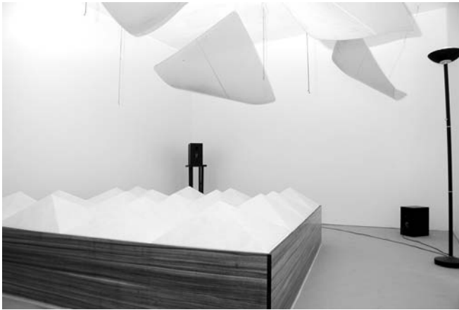
Figure 2.22 The small reverberation chamber at RPG Diffusor Systems, Inc. (Photo courtesy of RPG Diffusor Systems Inc.)
