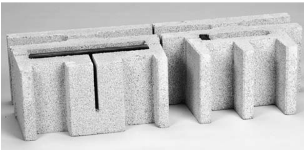
Figure 6.10 CMU (concrete masonry unit) which uses two slotted Helmholtz absorbers to provide bass absorption, DiffusorBlox ® (one slot is difficult to see).
