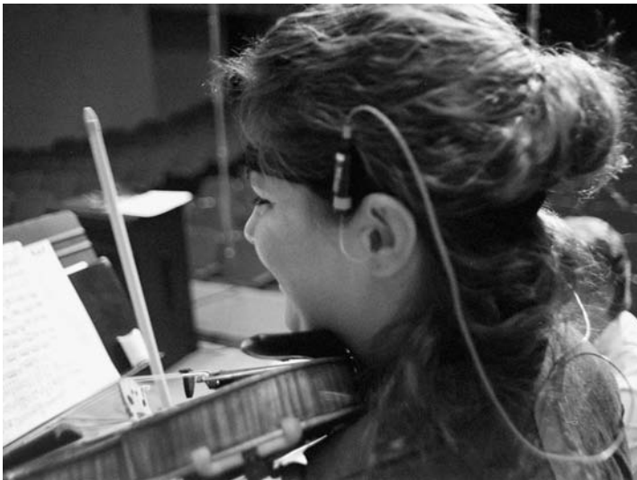
Figure 2.31 Probe microphone inserted into the ear canal of the first violinist. Microphone is inserted to a point just in front of the ear drum (after D’Antonio 29 ).
