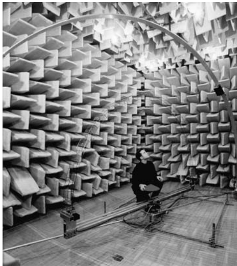
Figure 4.3 A system for measuring the scattering from a surface over a hemisphere. The diffuser being tested is the small pyramid in the centre. The source arc is most obvious, the receiver arc is acoustically transparent and so is difficult to see (reproduced from AES-4id-2001, with permission 2 ).
